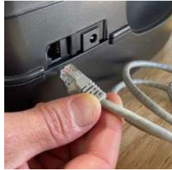
Fig. d: Plug transmitter into the back of the PRO base unit
